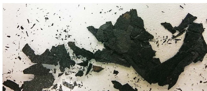
▲ Corrosion material from the inner pipewall which have not been sufficiently passivated and therefore corrosion arise.
