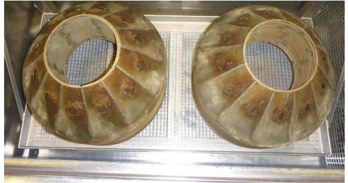
▲ Example of dishes ready to be cleaned and placed in a bath waiting for the ultrasound to be applied.
