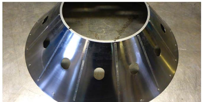
▲ After: The environmental friendly and effective cleaning has removed all unwanted particles and grease.
