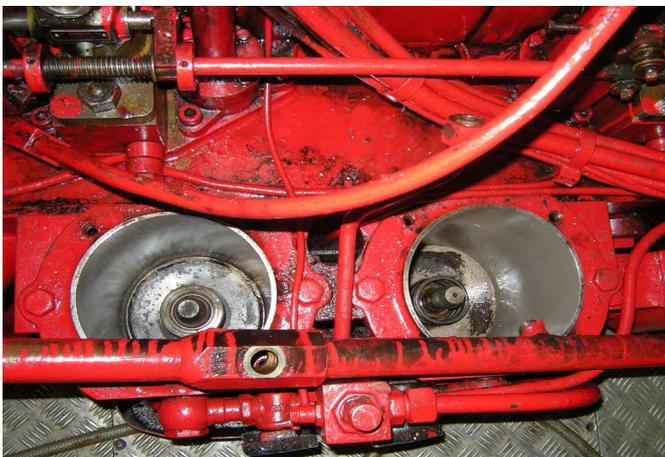
▲ Filterhouse Demounted for Cleaning
