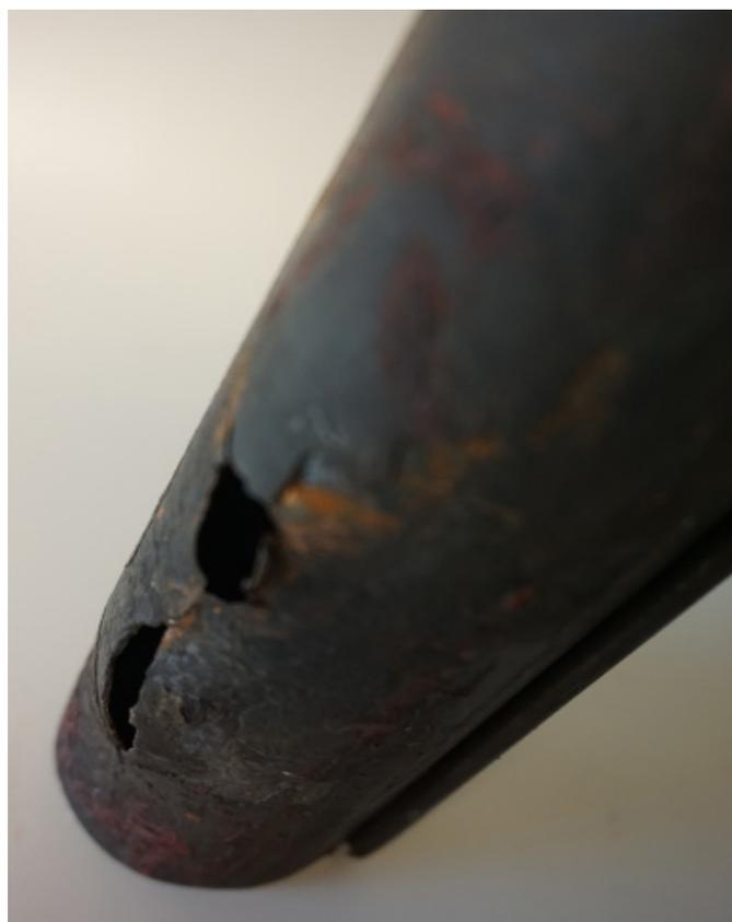
▲ Exploded Boiler Tube
