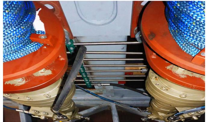
▲ Hydraulic motor for tensioning systems
