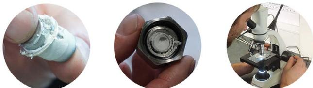
▲ Wax from pipe extruding is one of the results from cleaning a new "clean" umbilical with Liquid and Supercritical CO<sub>2</sub> Flush Technology
