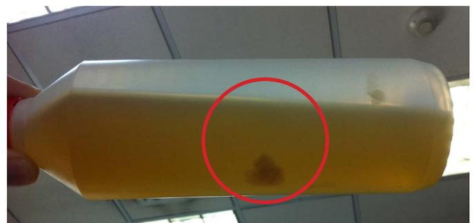
**Picture 2** – Clear worn out additives from an oil sample.
