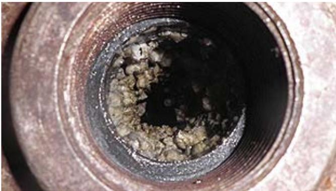
*Picture 1 – The two Alfa Laval plate heat exchangers were obviously strongly affected by mussels, snails and other types of marine fouling.*
