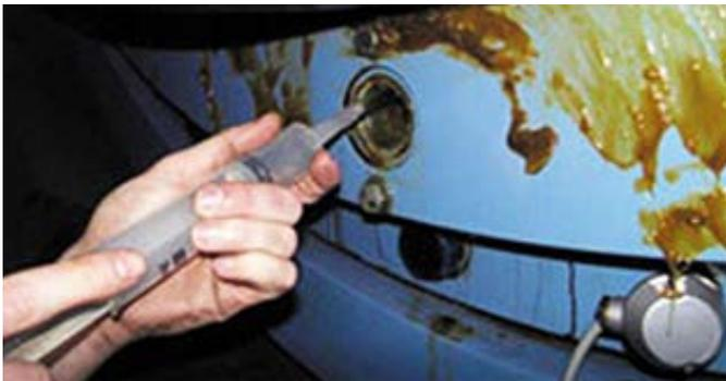
▲ *Picture of an over-greased bearing, where the fresh grease has been forced out of the bearing seals.*
