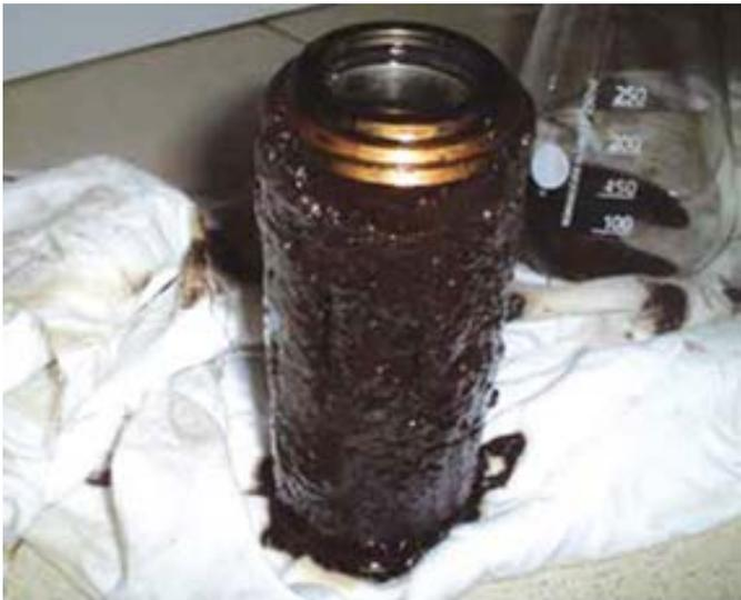
**Picture 1** – Plugged filter with remains of oxidation from a large-frame industrial gas turbine.
