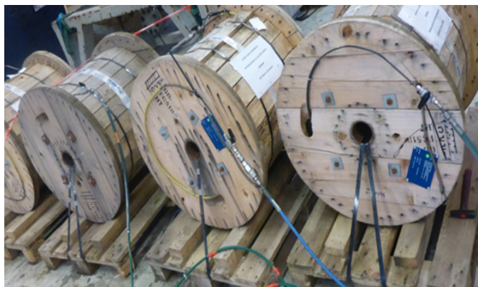
▲ 4 x 1/4" OD x 0,049" wall, L: 2400 Ft, Nickel based Alloy 825
